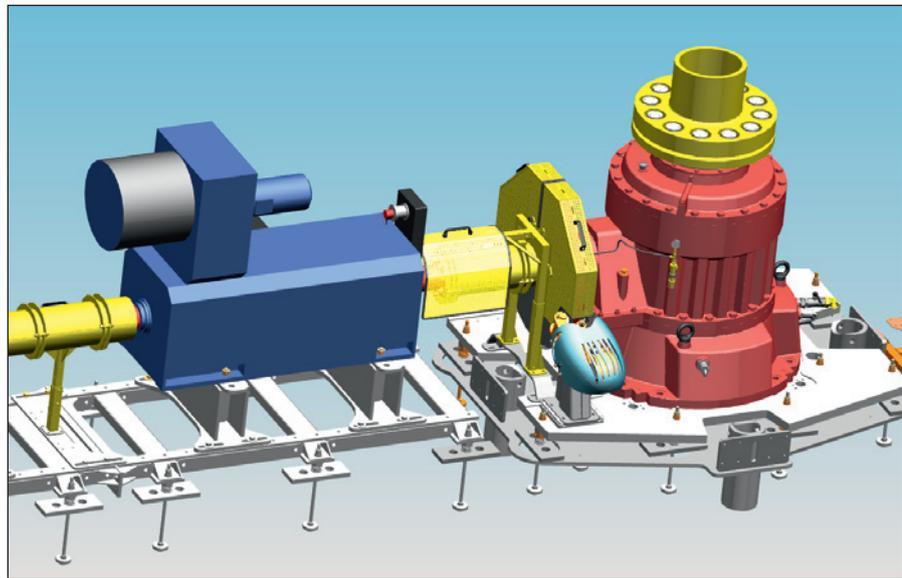
**Benefits** The underground set-up of electric motor and gearbox ensures **low noise emissions** in the station area and **maximum protection** of the drive components **at low temperatures**.
