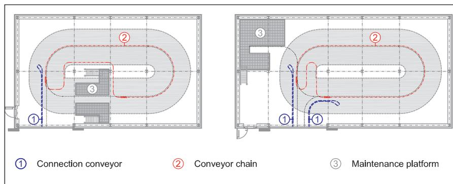
**Benefits** If the rail switch system is set accordingly, **each vehicle** can be brought **individually to the maintenance platform**. During maintenance, all vehicles can remain in the parking building. **Inspections and maintenance** can therefore be performed **without** having to **consider** the **weather conditions**.
